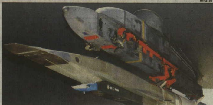
NEED FOR SPEED: A US Air Force B-52 (top) carries the X-51 WaveRider for a test flight. The special plane is being developed to strike targets super-fast
